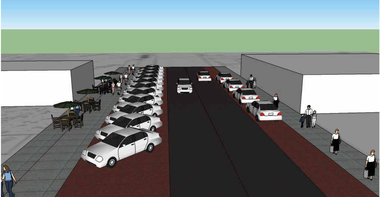
3D computer illustration of First Street looking west from North Portage Birdseye view of proposed parking and sidewalk layout from the Concept Layout Plan (Figure 2).
